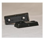
11050 7/8" x 2-1/2" x 3/8" (13/32" recess) 5/32" holes 11050C (concave) 5/8" x 2-1/2" x 3/8" (13/32" recess) 5/32" holes
